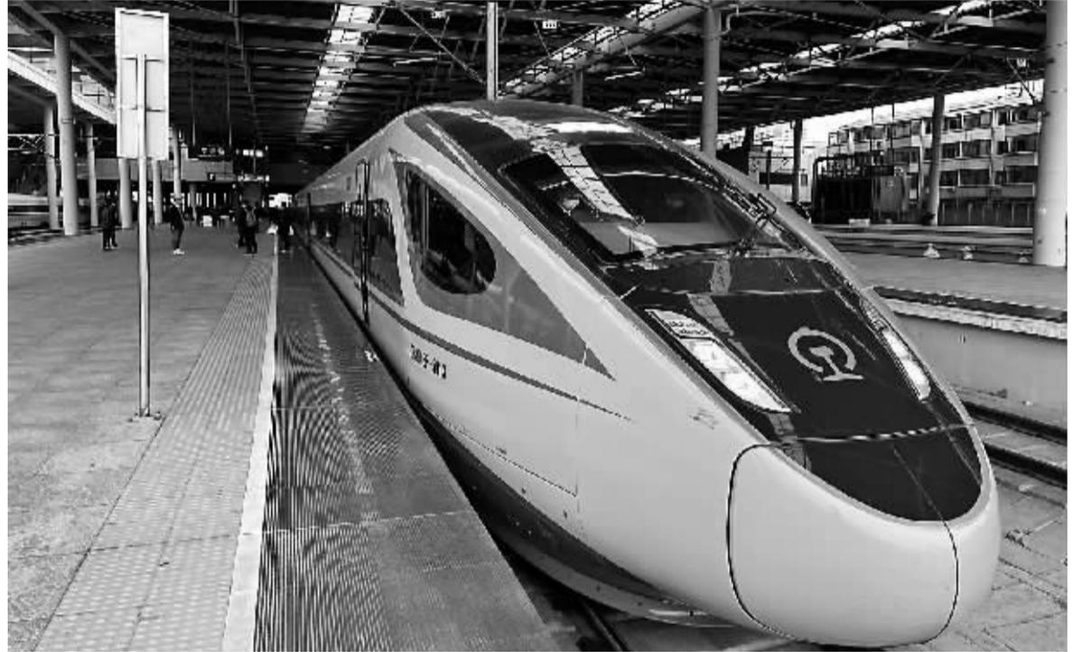
signed to run at a speed of 250 kilometers per hour, it has a seating capacity of 613, among which 48 are first-class seats and 565 second- class seats. When necessary, the CR300BF can be adjusted to the mode of coupled running, doubling its transport capacity.
